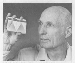
A SAMPLE of aluminum, cut in half, demonstrates how Lynn's Fractometer machine works — it applies a load to a material, cracks it open, and takes measurements during the process.
